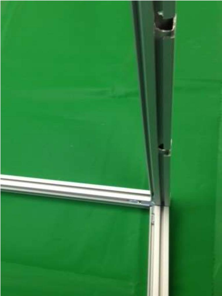
12. The next two 35" aluminum tubes to be installed will be the one with the two small holes drilled at each end and the one with the magnet attached, also with two small holes drilled at each end. Before installing these two pieces, open the bag containing the hinges and insert the black plastic grommets into the holes on each piece. You may need to tap them into place with a hammer.
