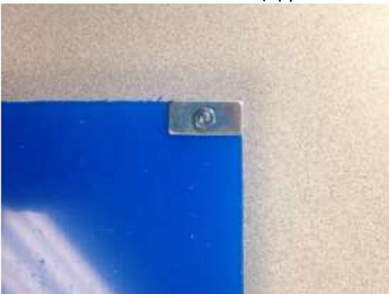
23. Place a hinge in the bottom hole and insert Plexiglas door, while holding door place a hinge in top hole and move door into top hinge. Lightly tighten screws to hold door in place.
