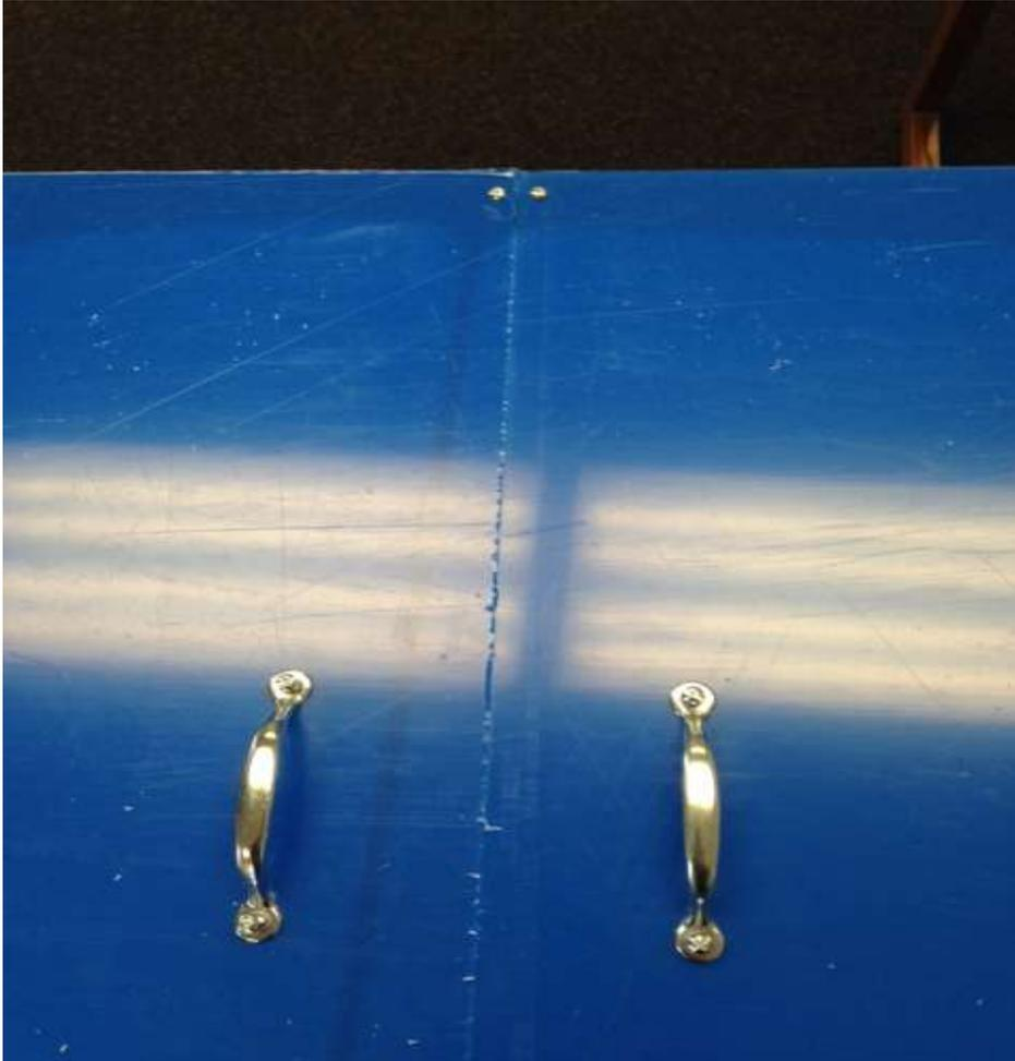
22. Place another machine screw into the single hole at the top of the door and attach a magnet catch on the inside of the door (opposite side of the handles).
